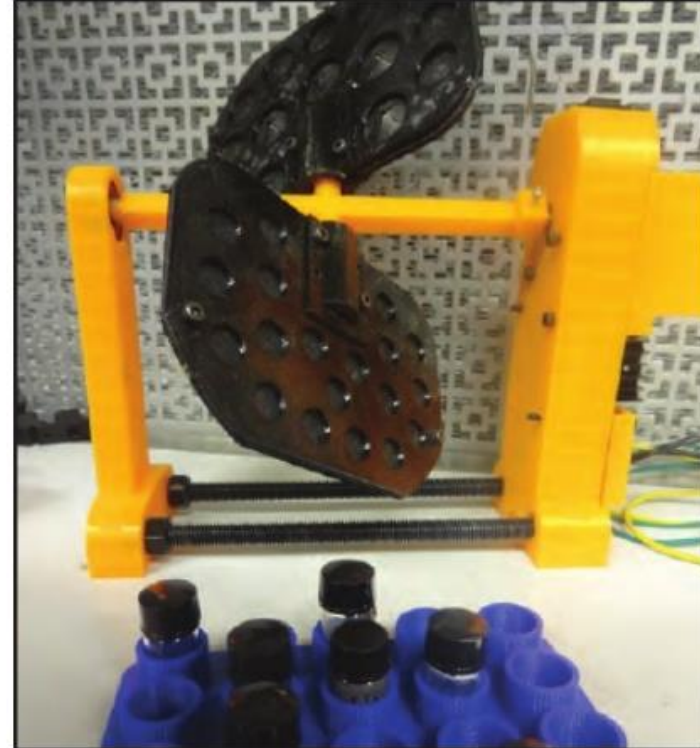
FIGURE 3 An open source 3D-printed sample holder and laboratory sample rotator mixer and shaker controlled with an open source Adafruit pro trinket microcontroller (Dhankani and Pearce 2017).
